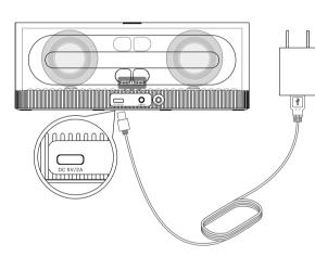
Connect USB - C charging cable to a power converter (Recommended 100V - 240V) and SB-X200 as shown. Charging time - Approx. 3.5 Hours Playback time - 8 Hours (Dependent on playback volume)
