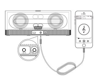
Line-In - (External audio source) Power on, connect external audio source and SB-X200 via 3.5mm AUX Cable.
